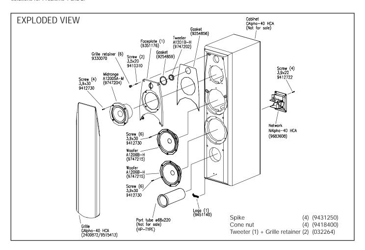
Note: A Phillips screwdriver and "Torx" bit screwdriver T20 size are required to service this product
